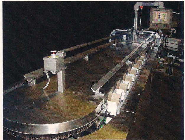
NEW CARTONER. New controls technology helped Ultra Packaging build a cartoning machine that offers greater flexibility, faster changeover, and reduced wiring and maintenance. Footprint is smaller, too.
